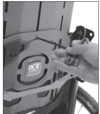
Fig. 6: Loosen 3 cap screws to adjust back height
